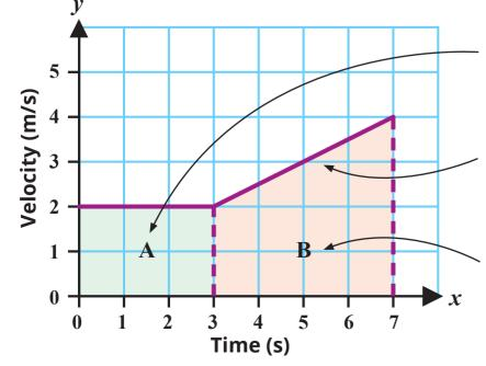
distance of  $3 \times 2 = 6m$  was travelled at a constant velocity of 2m/s for 3s
